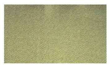
GC1000 FH1000 is a texturized E-glass fabric impregnated with a FH1000 treatment made from Vermiculite to improve resistance to abrasion and molten metals.
